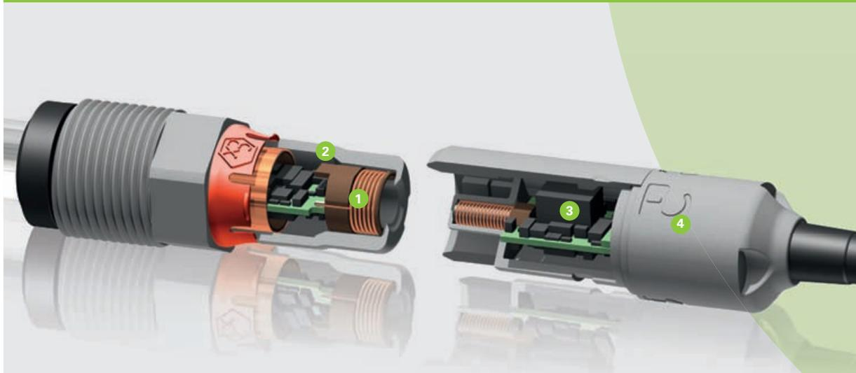
1 The inductive connection supplies power to the sensor plug-in head and also enables bi-directional signal transmission between the sensor plug-in head and the cable coupling.
